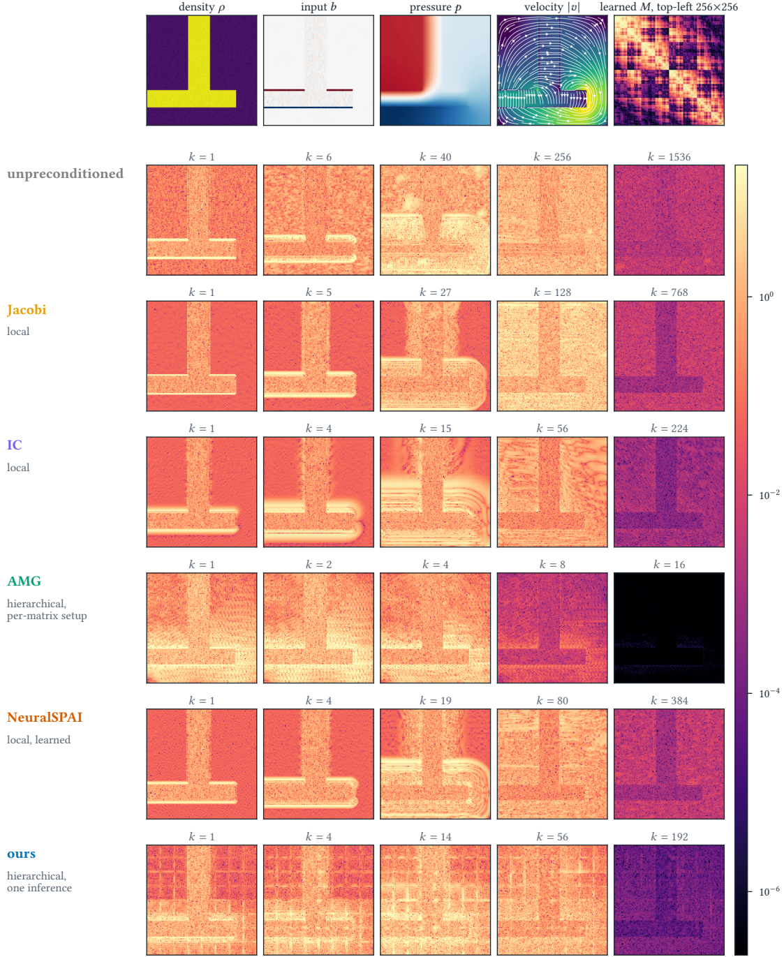
Figure 2: Residual magnitude |r_k| during PCG on a 2D multiphase Poisson frame at N = 16,384 . Top strip: density, right-hand side, pressure, velocity and the learned M . Each row is one method, labelled with its kind, shown at five iterations k on its own schedule.
